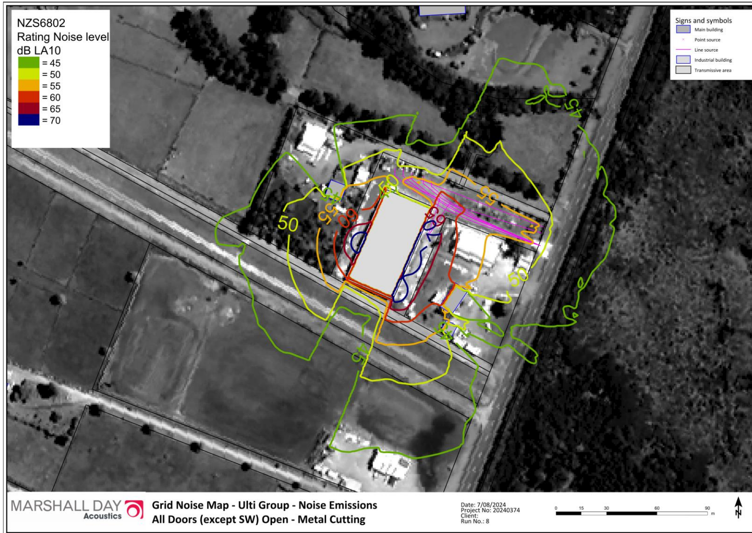
Figure 3: All Doors Open (excluding SW doors)
