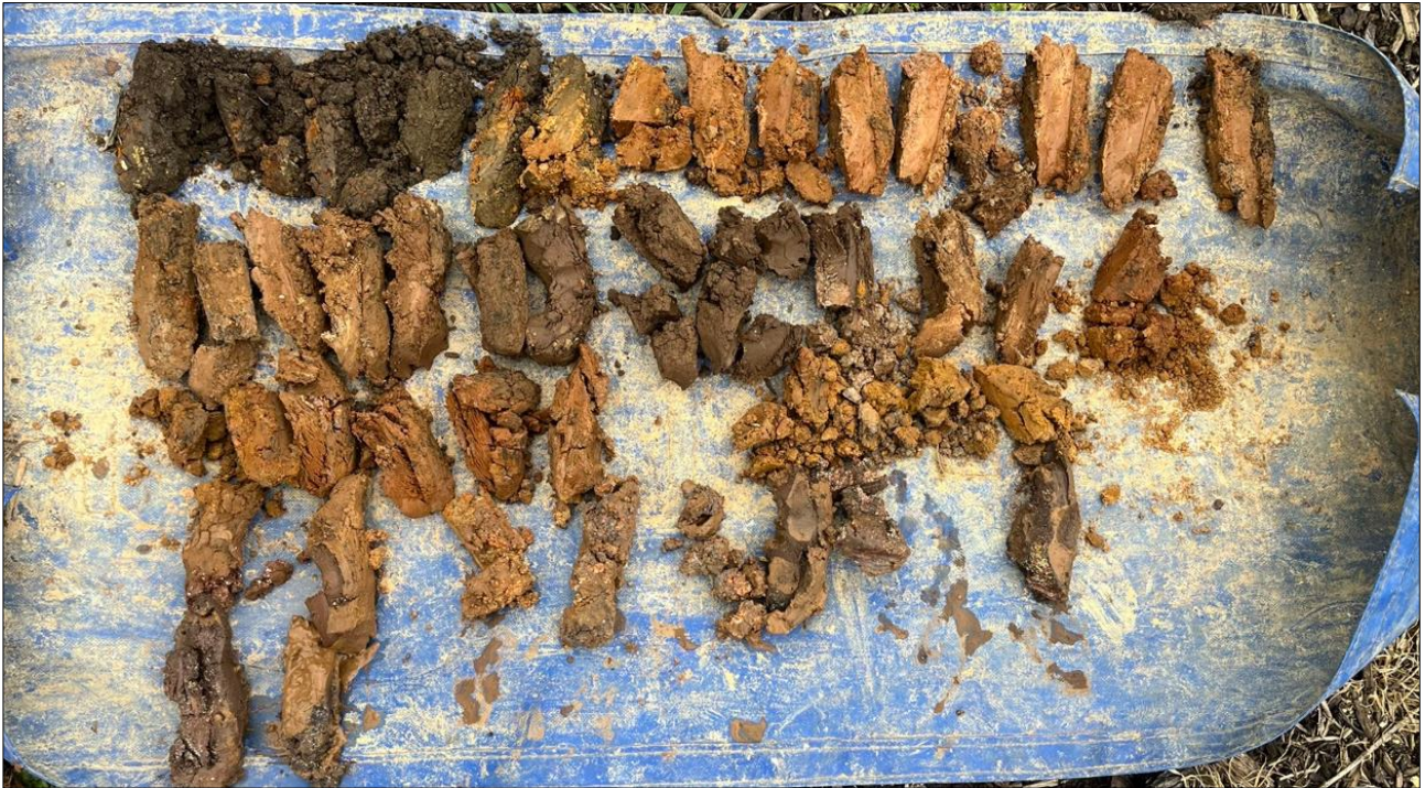
Figure 8: Site photograph of the HA01 soil arisings (0.0m to 4.8m).
