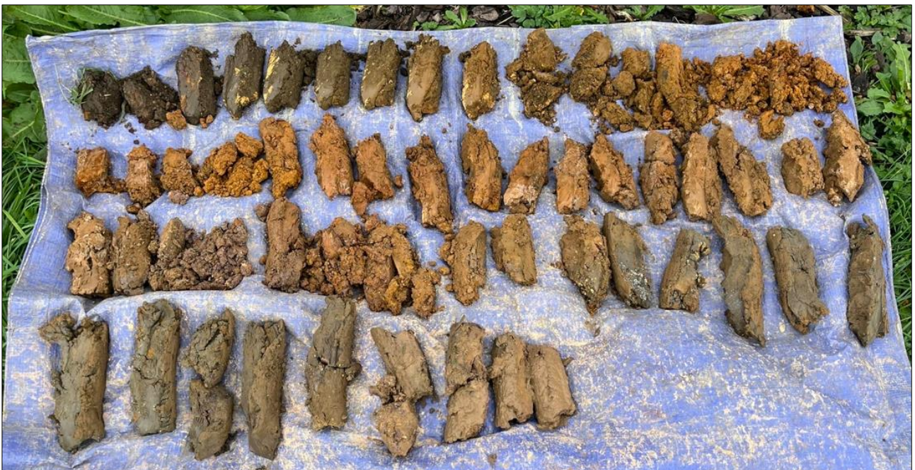
Figure 9: Site photograph of the HA02 soil arisings (0.0m to 4.5m).
