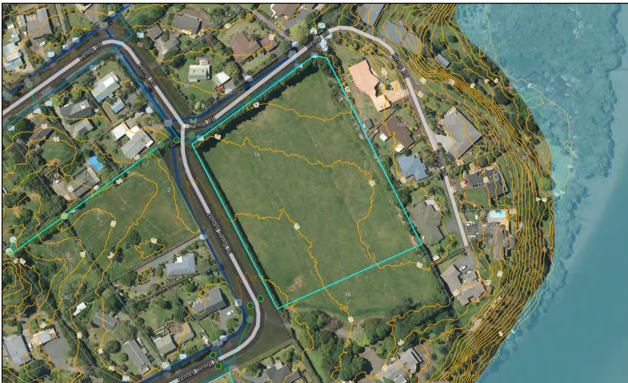
Figure 2: Screenshot Aerial View of the Site from FNDC GIS Water Services Map Showing Site Boundaries (cyan), Public Stormwater (green), Public Potable Water (blue) and 1m Contours (yellow).
