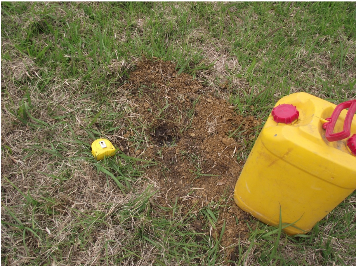
Close up view of the soakage test hole & soil removed.
