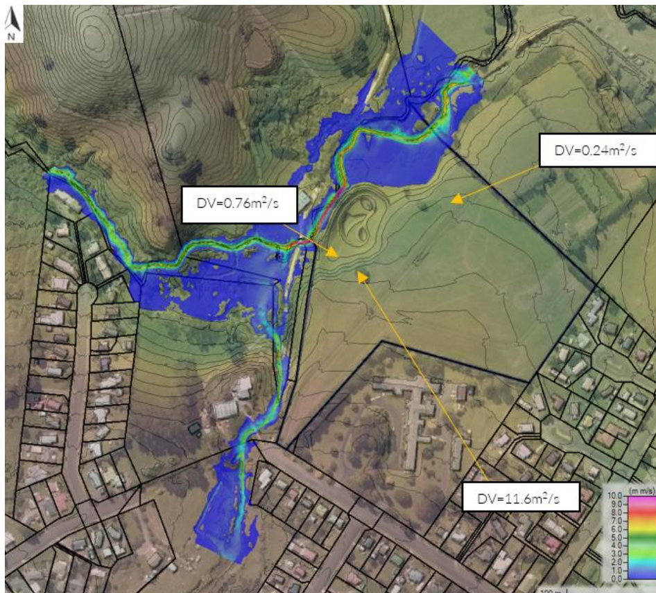
Figure 8: 1% AEP (MPD + CC) maximum flood depth x velocity from the post-development model
