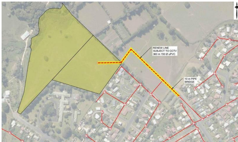
Figure 11: Bisset Road WW Line Renewal Works
