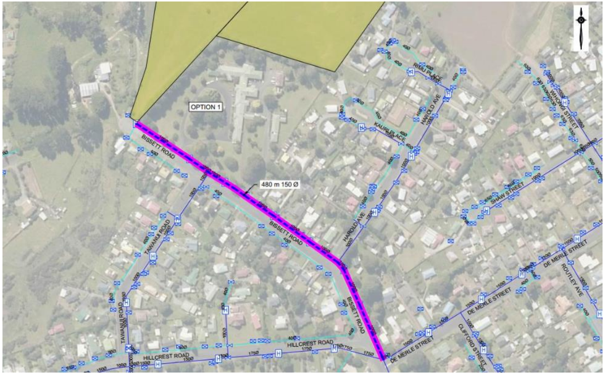
Figure 8: Bisset Road water main renewal works (Haigh Workman)
