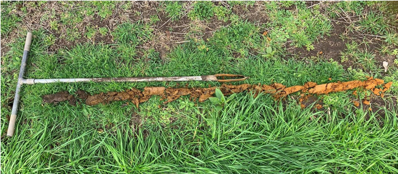
Photograph 2: Borehole showing 100mm of category 4, slightly moist, dark brown topsoil followed by category 5, slightly moist, orangey brown, silty clay to a depth of 700mm. From 700-1200mm soils were category 6, slightly moist, orange, silty clay.
