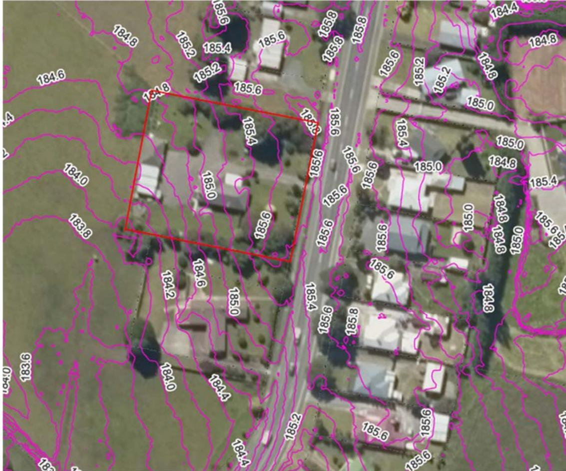
Figure 2: Existing site contours for 15 Guy Road from 2020 lidar data
