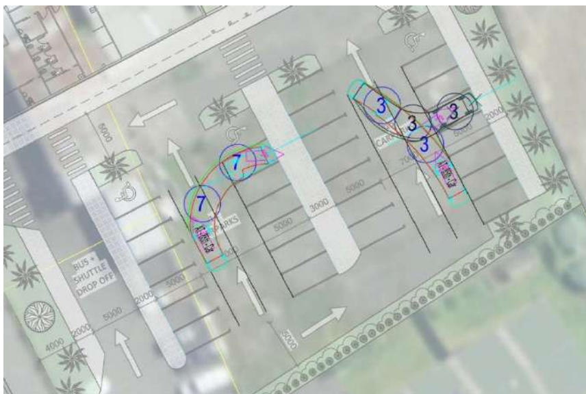
Figure 14 Snip of vehicle tracking for the car park using the 85 th percentile vehicle.
