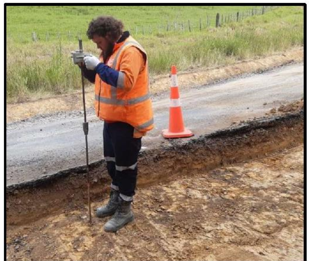
Shoulder check out (Left), Thorne carrying out Scala Penetrometer testing on a dig out.
