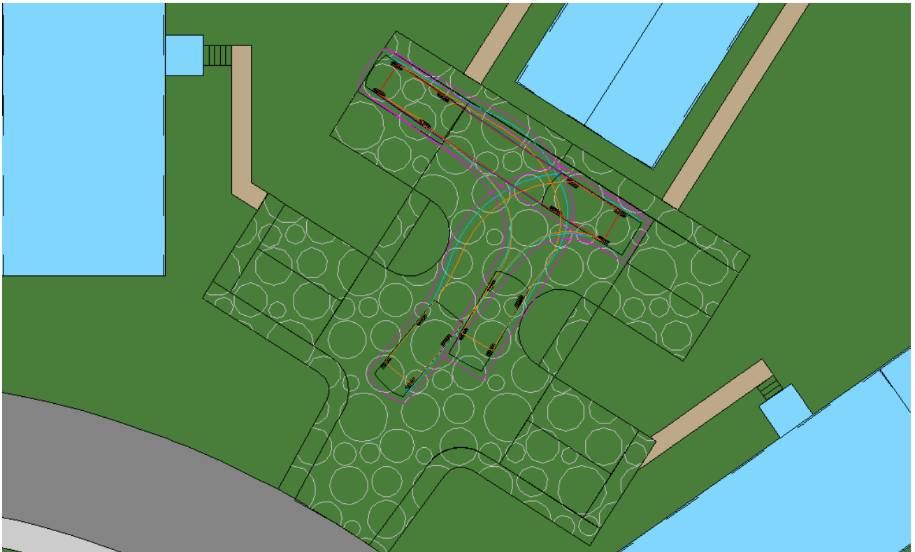
Figure 63: Road 2A- Unit 10a Parking Space 2 – 85 th percentile car.
