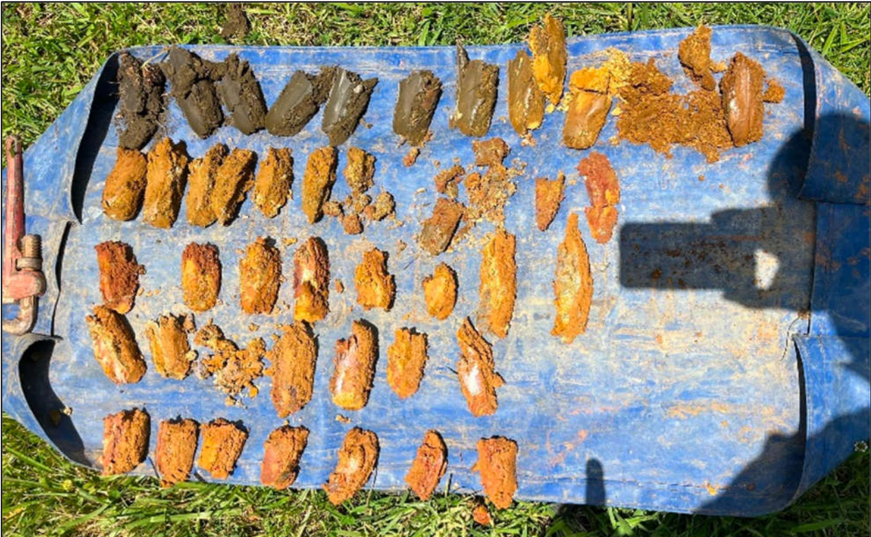
Figure 7: Site photograph of the typical HA soil arising encountered (HA01: 0.0m to 5.0m).
