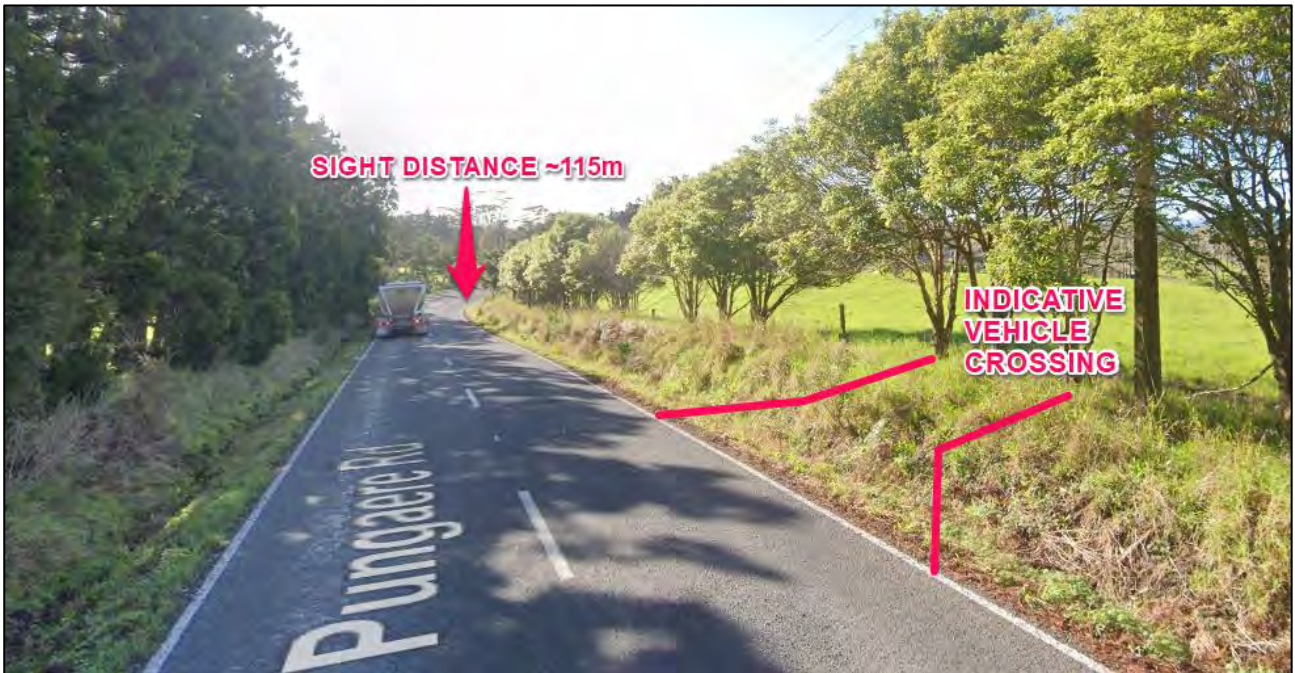
Figure 23 – Proposed Access Point on Pungaere Road Facing Northeast - ~115m Sight Distance Available
