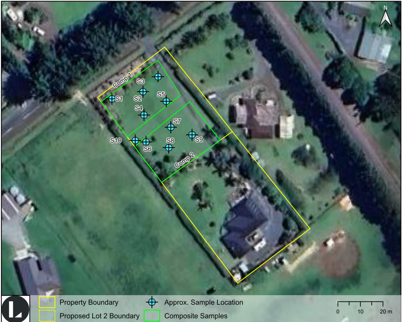
Figure 16. Soil sampling site plan. The approximate soil sampling locations are shown in blue and composite sample groups are shown in green. Source: Google Earth (annotated image).
