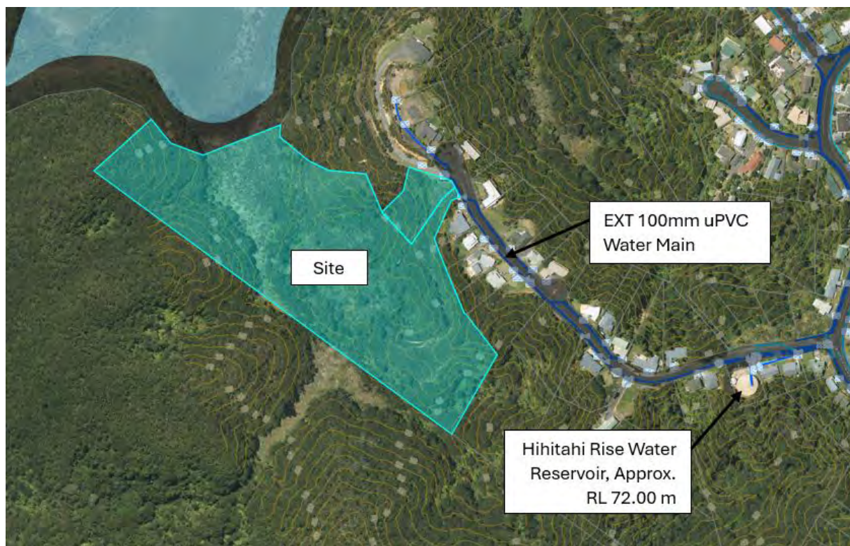
Figure 5: Existing Water Supply Network (FNDC Maps Accessed: 13/05/2024)
