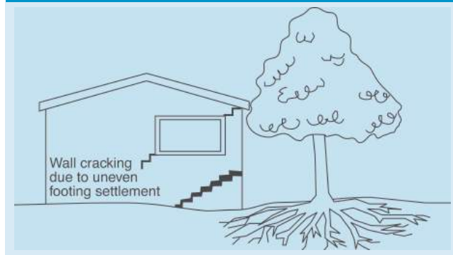
Trees can cause shrinkage and damage
