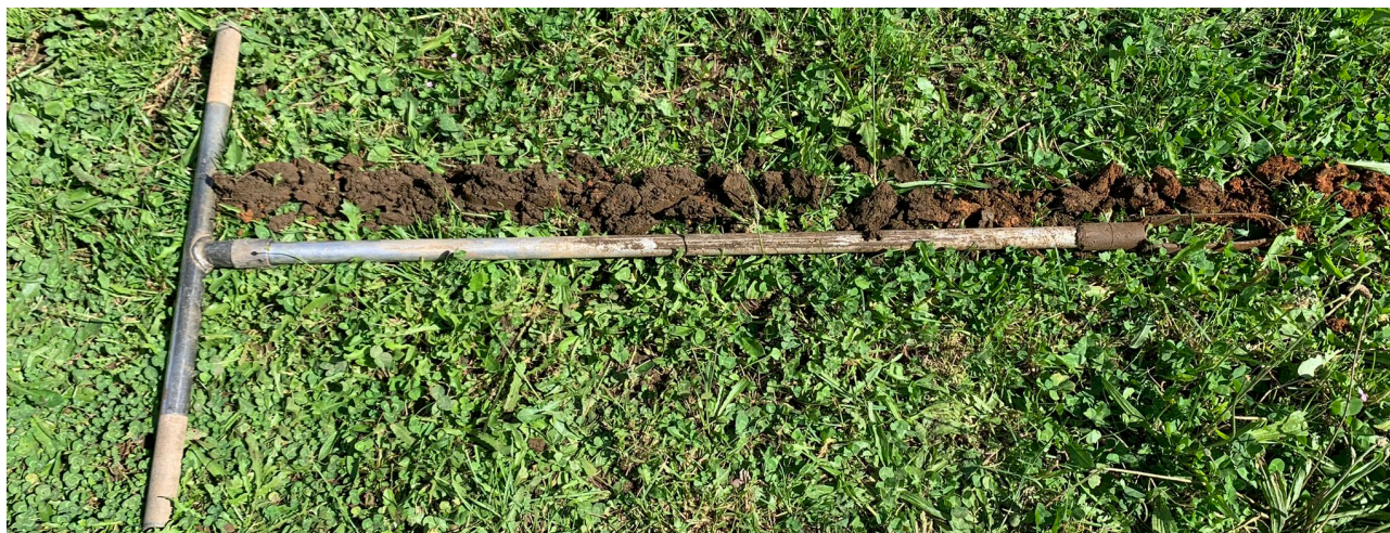
Photograph 2: Borehole showing 250mm of category 4, slightly moist, brown topsoil followed by category 4, slightly moist, brown silty clay loam to a depth of 800mm. From 800-1200mm soils were category 5 gravelly, friable, clay loam.
