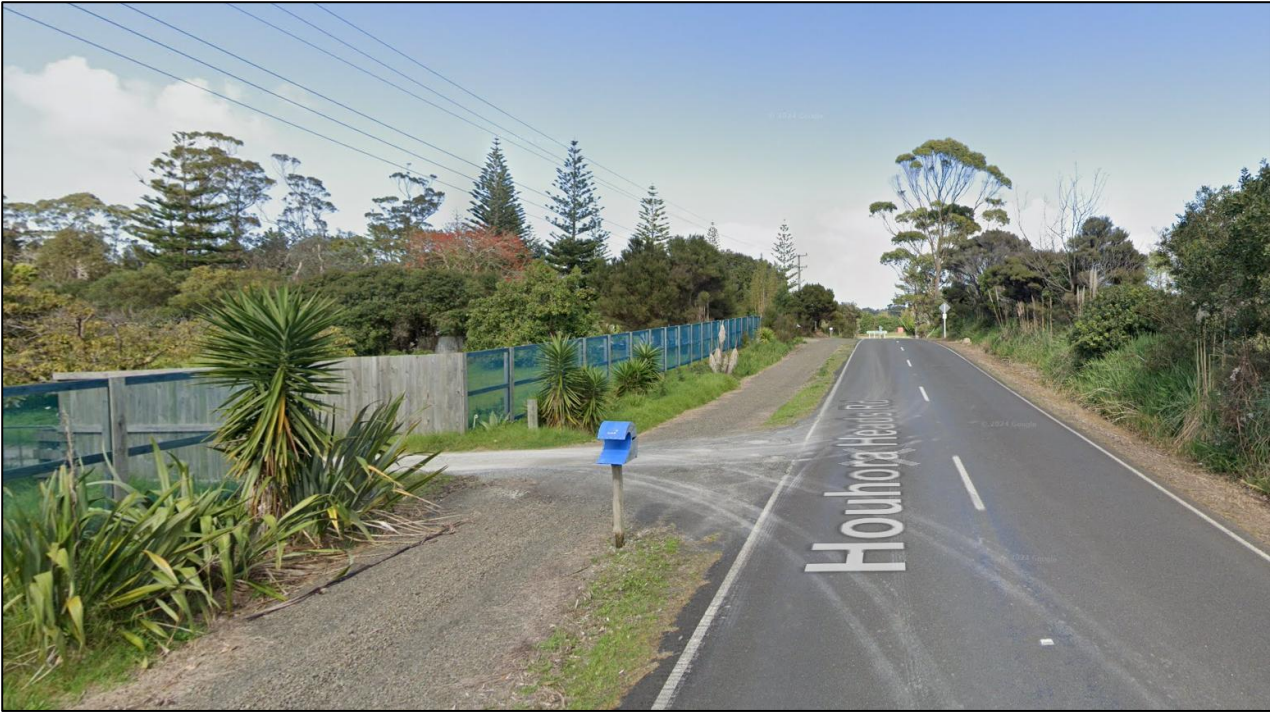
Figure 15: View of existing northern access point on Houhora Heads Road facing southwest, estimated 87m sight distance available due to local high-point obstruction.
