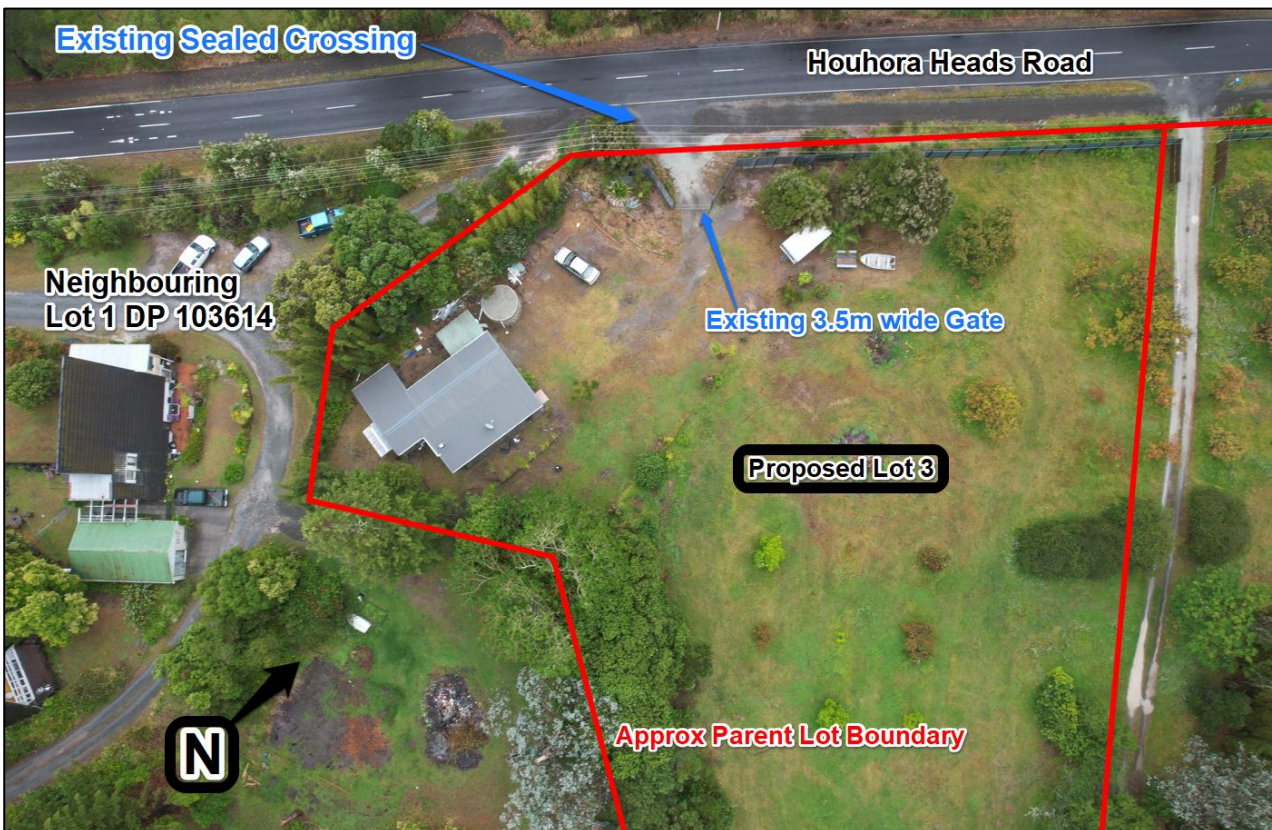
Figure 8: Drone Aerial Photo 15.11.2024 - Markup showing existing crossing and gate serving house on S3 Proposed Lot 3.
