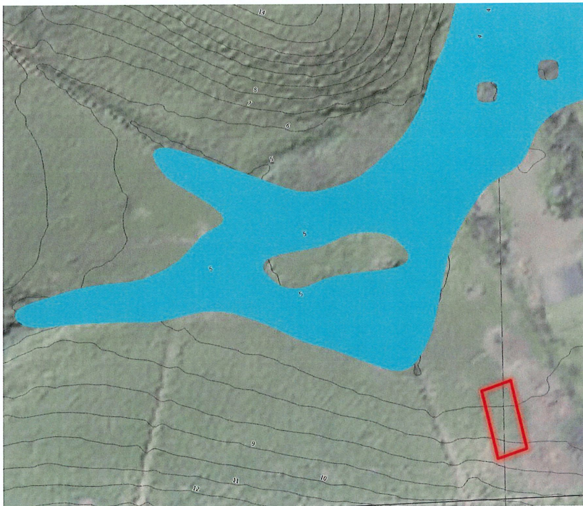
Figure 3. NRC Regionwide Flood Model for 100 year ARI + CC Approximate relocatable Dwelling Location in red, Flood extent in blue.
