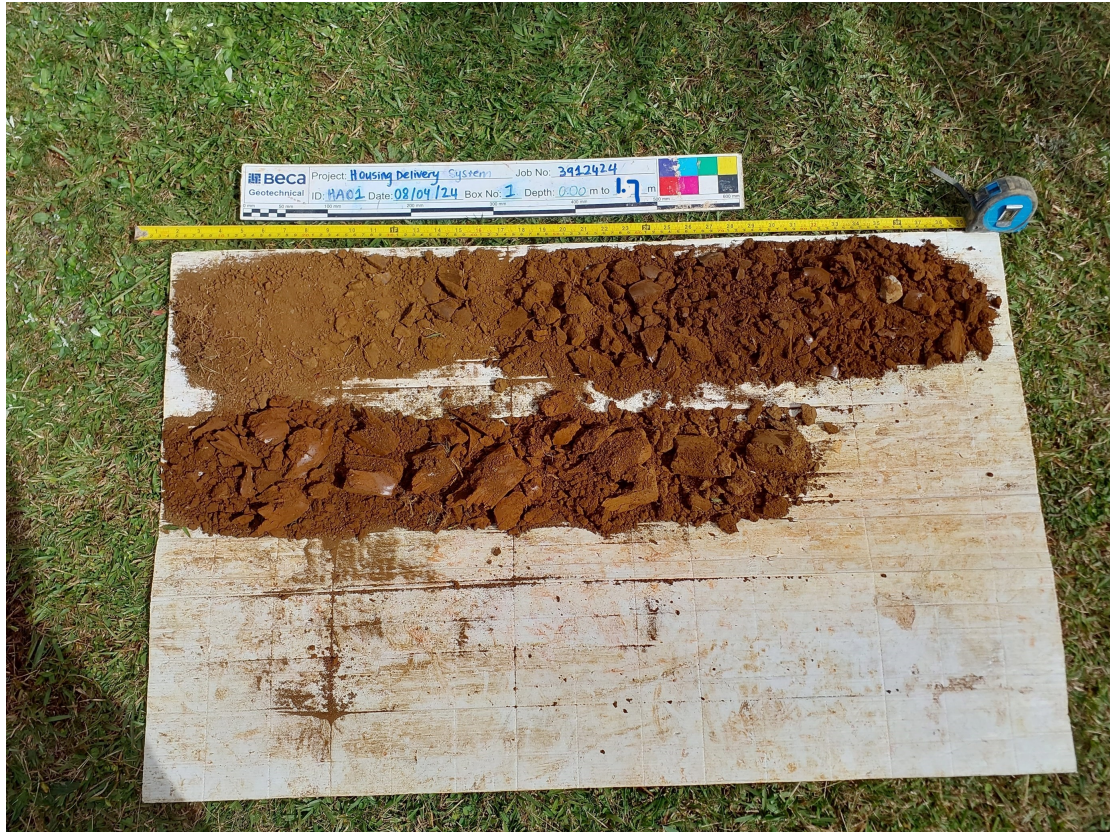
Box 1 - 0.00mbgl to 2.70mbgl
