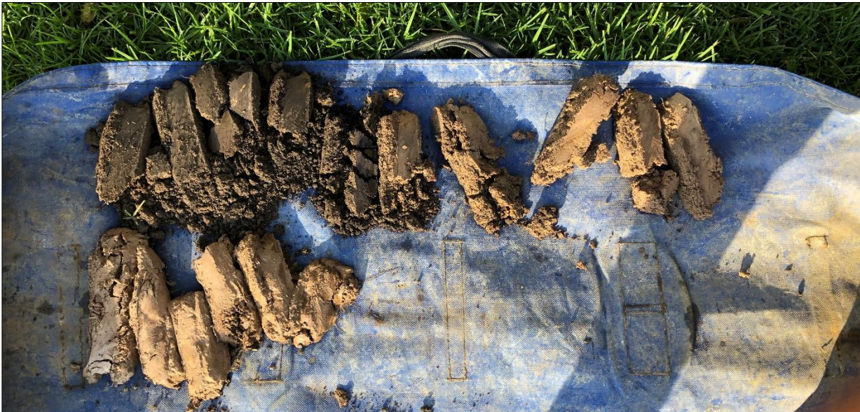
Figure 9: Site photograph of the typical soil arisings (HA01: 0.0m to 1.5m).
