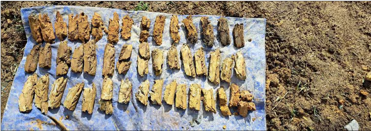
Figure 8: Site photograph of the HA02 soil arisings (0.0m to 4.0m).
