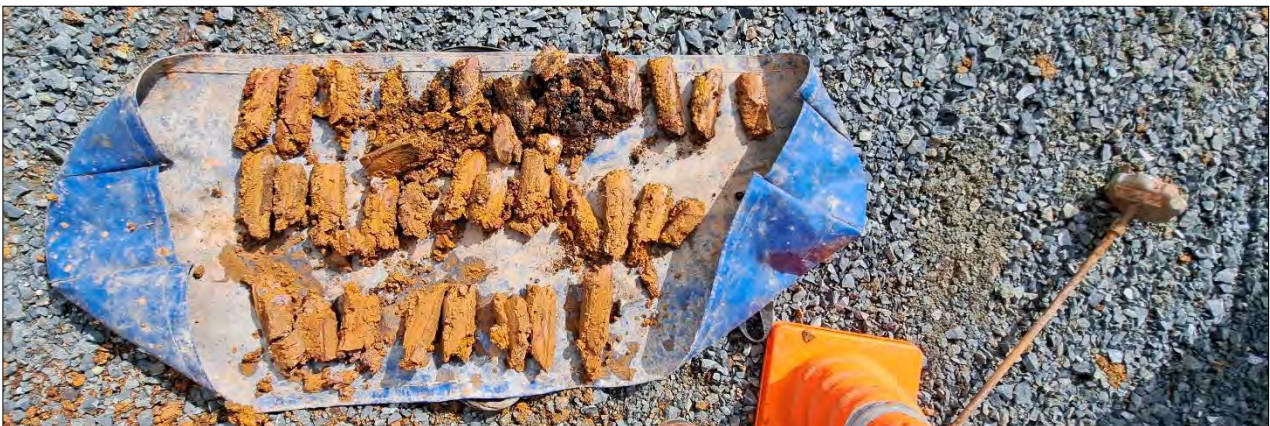
Figure 7: Site photograph of the HA01 soil arisings (0.0m to 3.0m).
