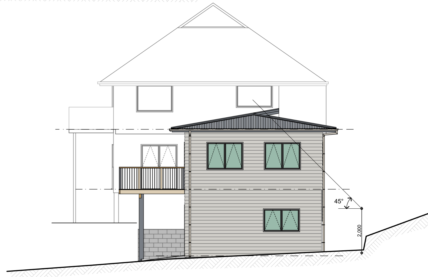
02 West Elevation Scale 1:100
