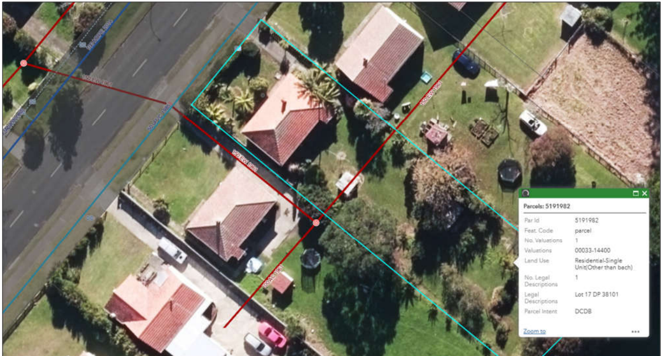
Figure 4: Screenshot aerial view of the subject site from the FNDC on-line GIS Water Services Map. Property boundary is highlighted in cyan. Blue line is water, red line is wastewater.
