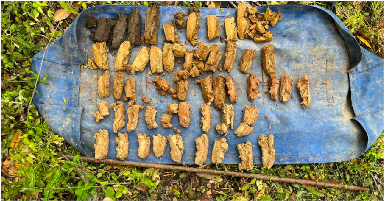
Figure 10: Site photograph of the HA06 soil arisings (0.0m to 5.0m).
