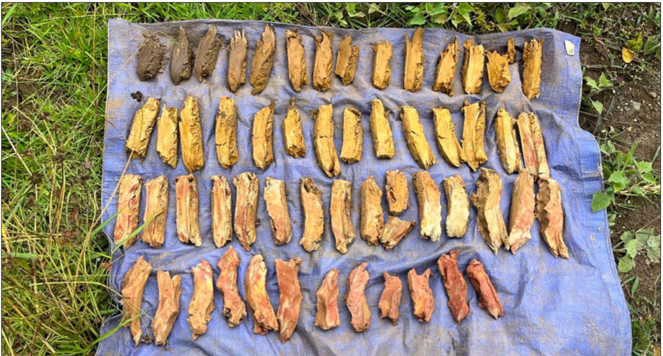
Figure 9: Site photograph of the HA01 soil arising (0.0m to 5.0m).
