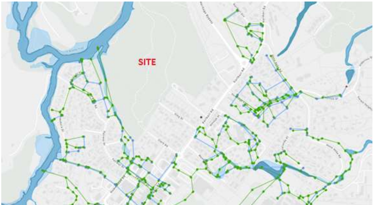
Figure 7 – Existing overland flowpath captured in FNDC Maps
