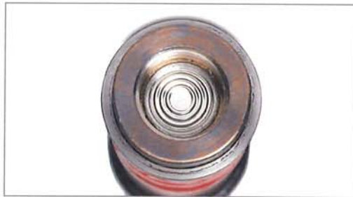
Figure 3 - U sensor properly cleaned
