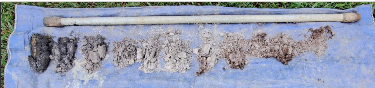
Figure 9: Site photograph of the typical HA soil arisings encountered on-site.
