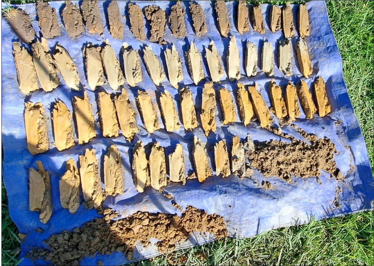
Figure 16: Site photograph of the HA02 soil arisings (0.0m – 4.6).
