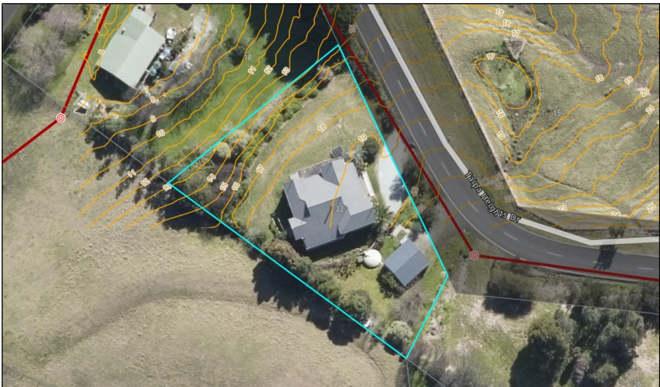
Figure 1: Aerial Snip (outdated satellite imagery) from FNDC Maps Showing Site Boundaries (cyan), Public Wastewater (red) & 1m Contours (yellow)
