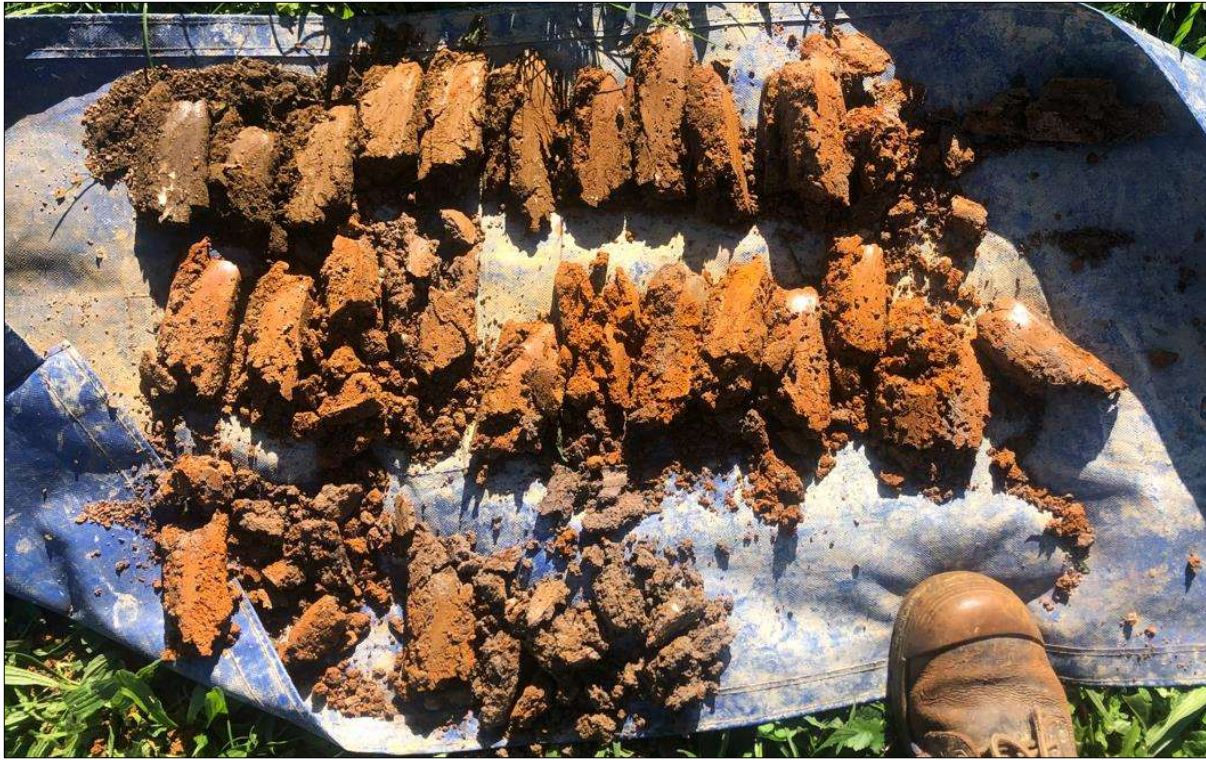
Figure 9: Site photograph of the typical HA soil arisings (HA01: 0.0m to 3.0m).
