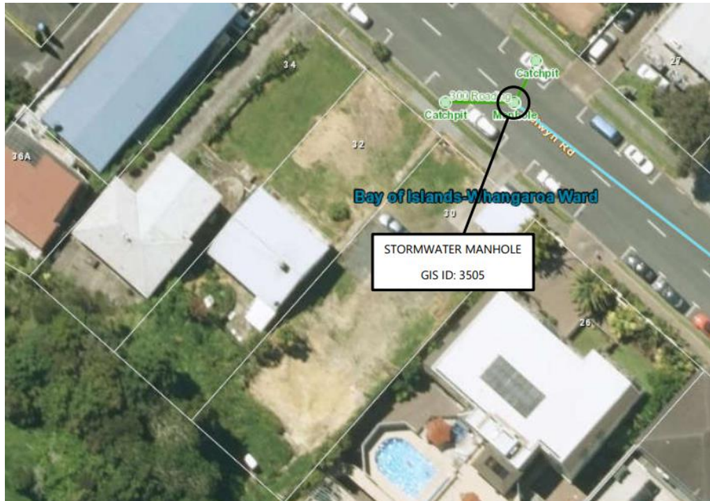
Figure 4: Existing Stormwater Network Layout
