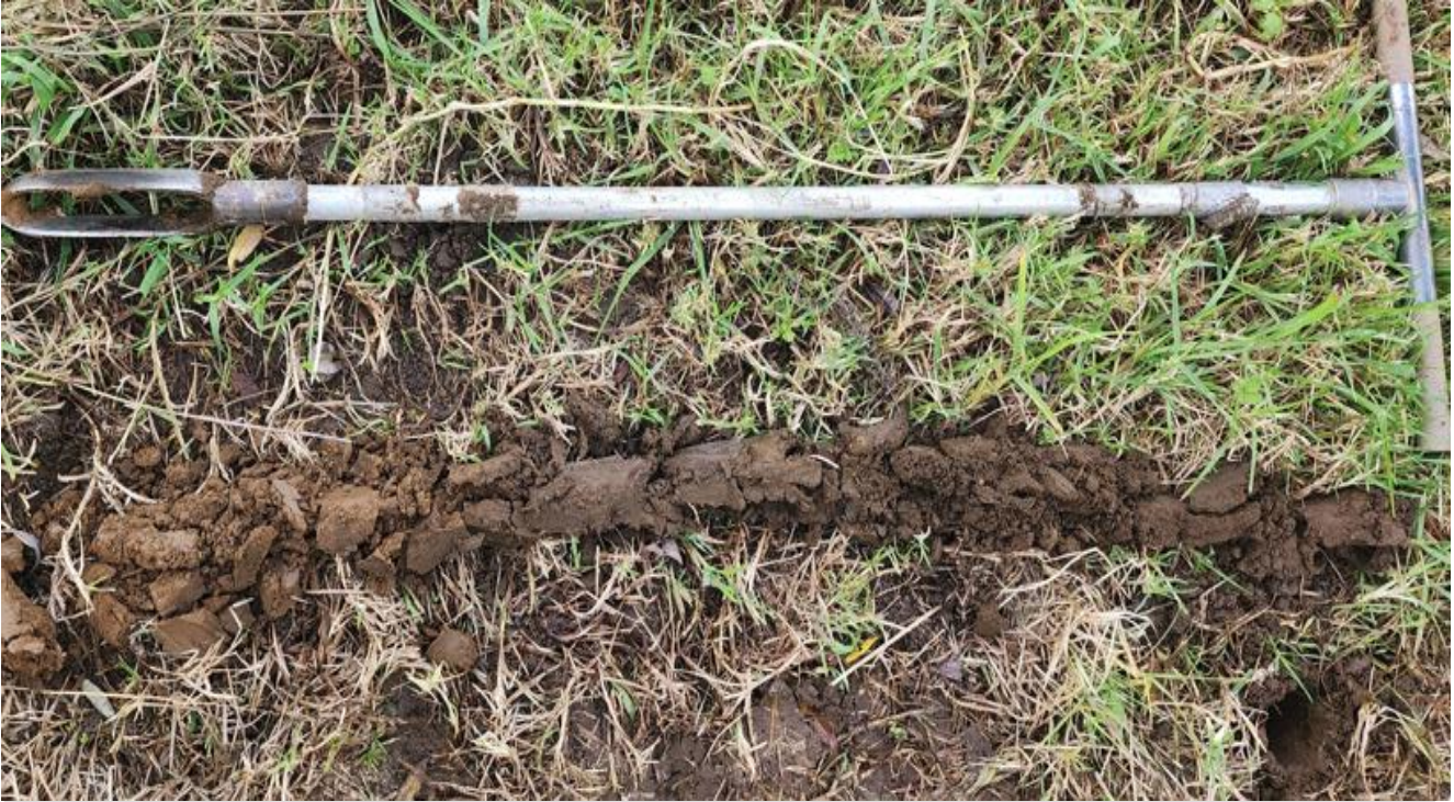
200mm topsoil over silty clay Class 6, (as per AC TP-58, Table 5.1)
