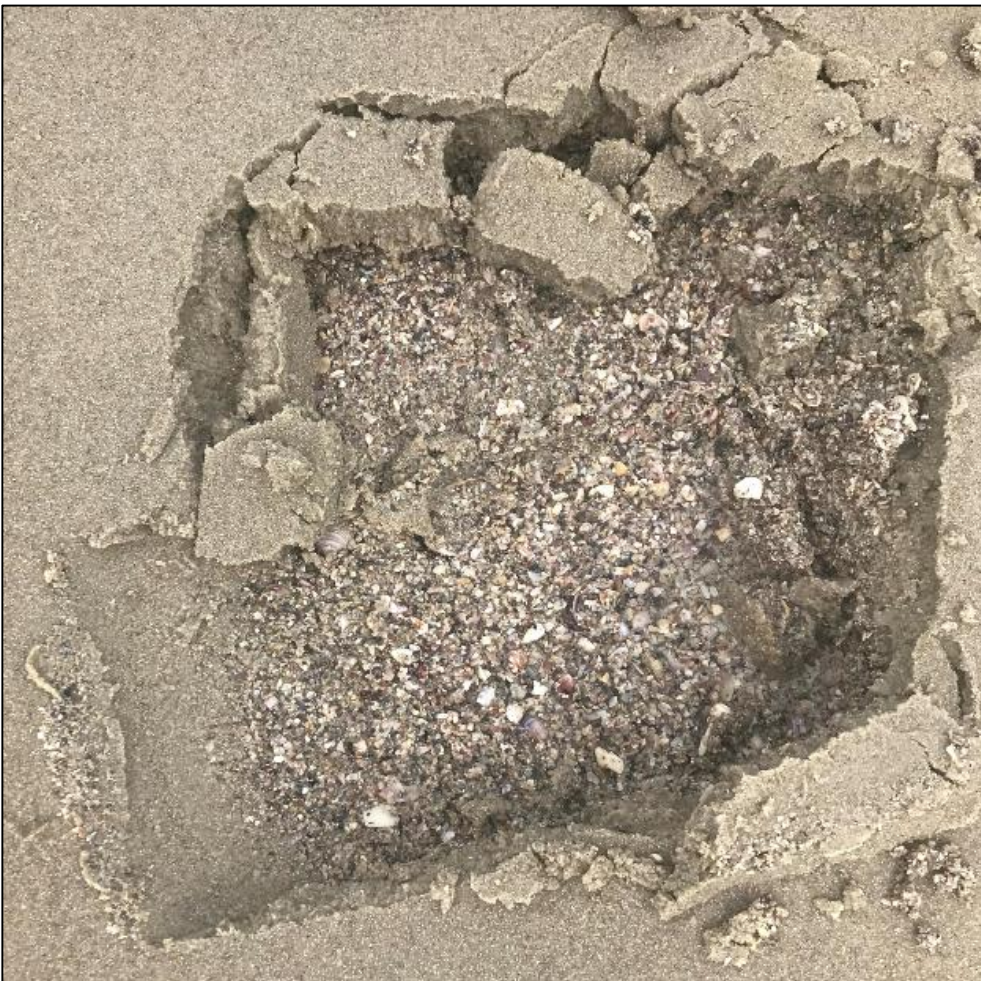
Site Photo 5: Distinct shell layer encountered around the 40m transect line, approximately 50mm below the surface. Photo taken 10 December 2020.
