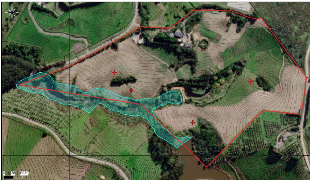
Figure 9: Indicative dam breach inundation map. Indicative inundation zone shown in blue shading. Proposed building locations shown as red crosses.
