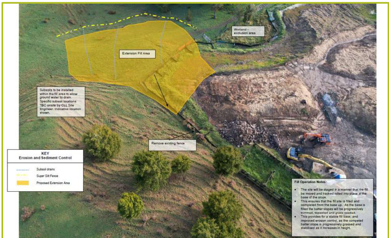
Figure 16: Snip from Erosion and Sediment Control Plan Showing Extension Fill Area, being Stage 3 (Source: Erosion and Sediment and Control Plan)
