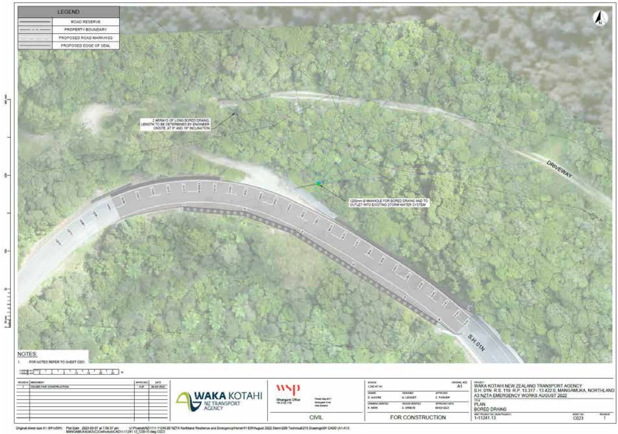
Figure 5: Slip A3, plan of bored drains.
