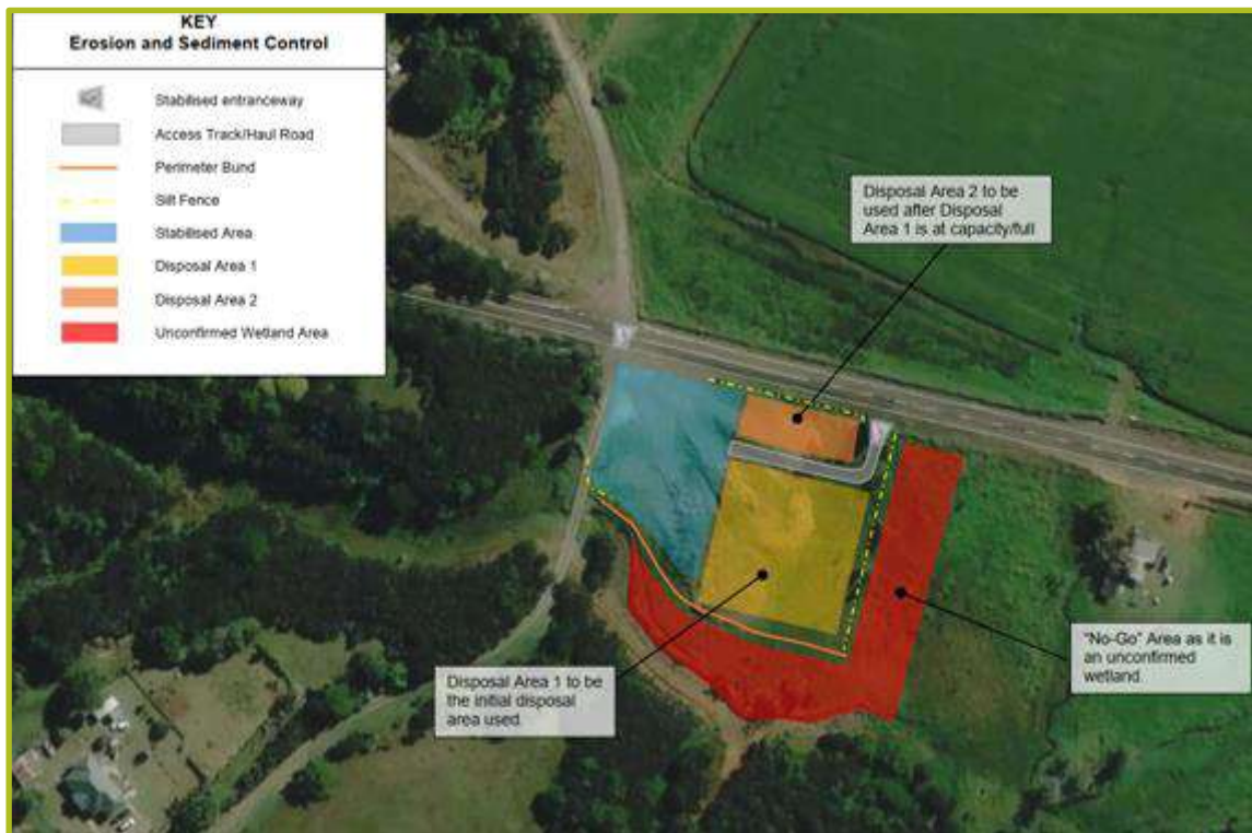
Figure 12: Excerpt from CLL Erosion & Sediment Control Plan, which also indicates “no go” zone in and around a natural inland wetland. Note that fill was not disposed on the site despite the notations on the plan. (Source: CLL Contractors)
