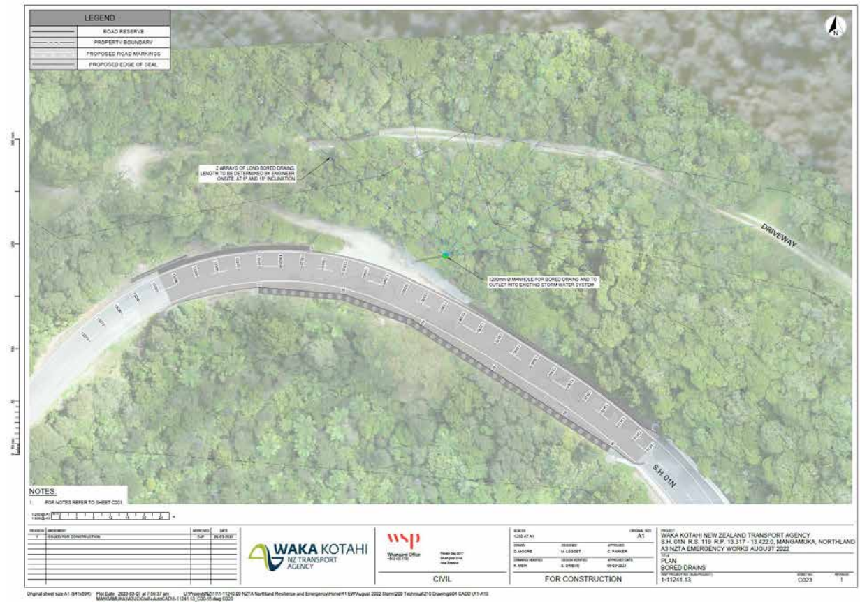
Figure 5: Slip A3, plan of bored drains.
