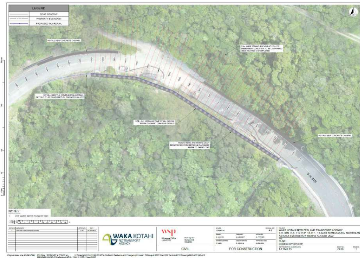
Figure 3: Slip A3, plan of concrete cap and pile retaining and new channelling.
