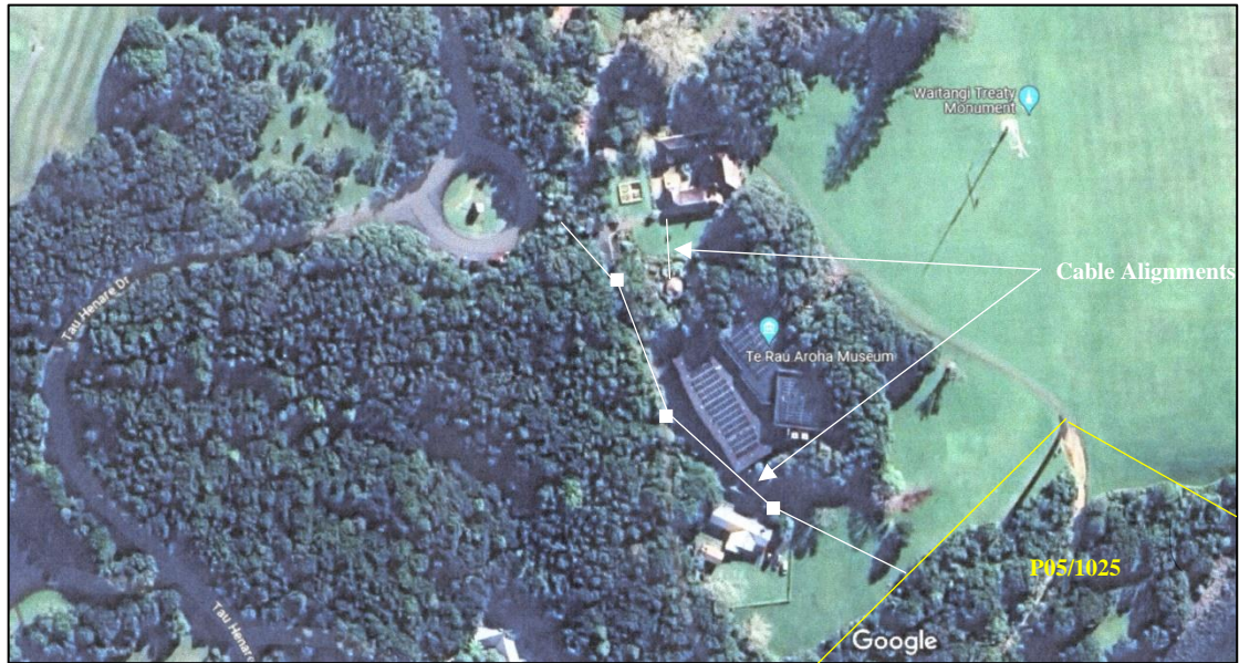
Figure 4: Upper Grounds with cable route (white) and approximate locations of jacking pits - white squares (Prince 2023 fibre route from Northcom plan).
