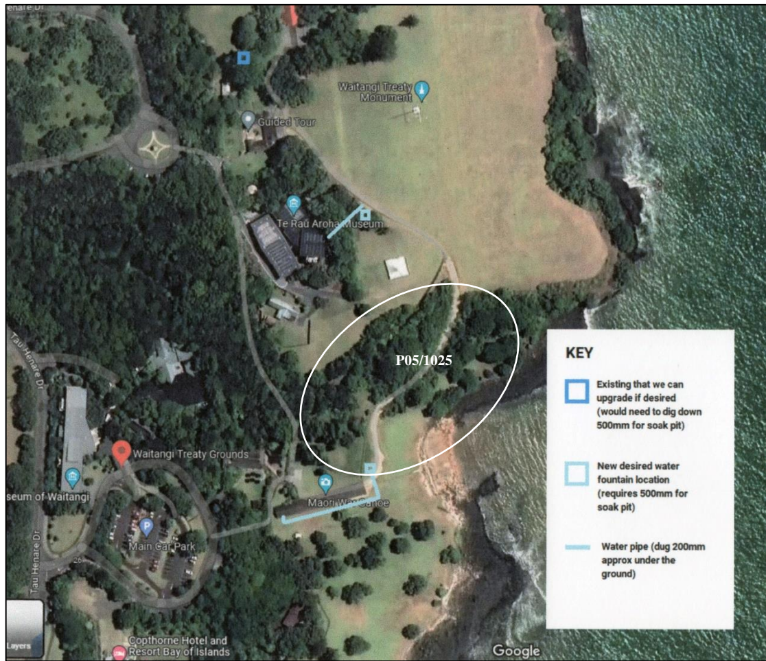
Figure 7: Proposed drinking fountains upgrade showing approximate extent of P05/1025 (Total Plumbing & Gas May 2023).
