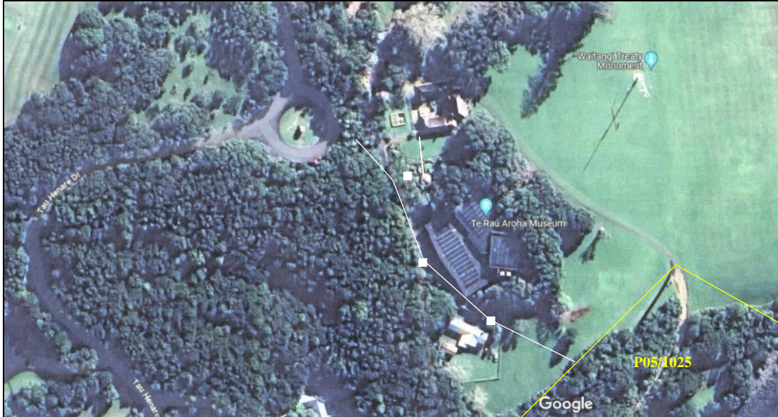
Figure 1: Upper Grounds with cable route (white) and approximate locations of jacking pits - white squares (Prince 2023 fibre route from Northcom plan).
