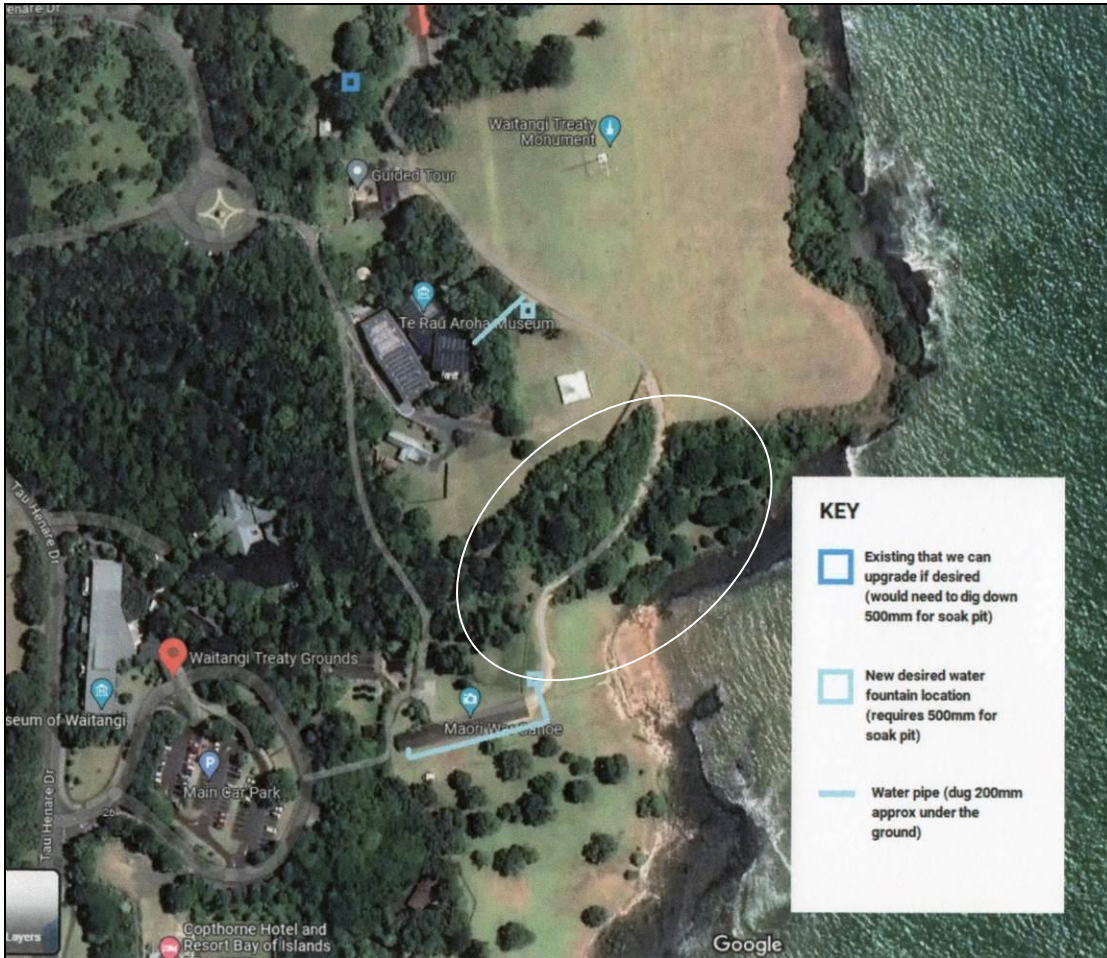
Figure 3: Proposed drinking fountains upgrade showing approximate extent of site P05/1025 (Total Plumbing & Gas May 2023).
