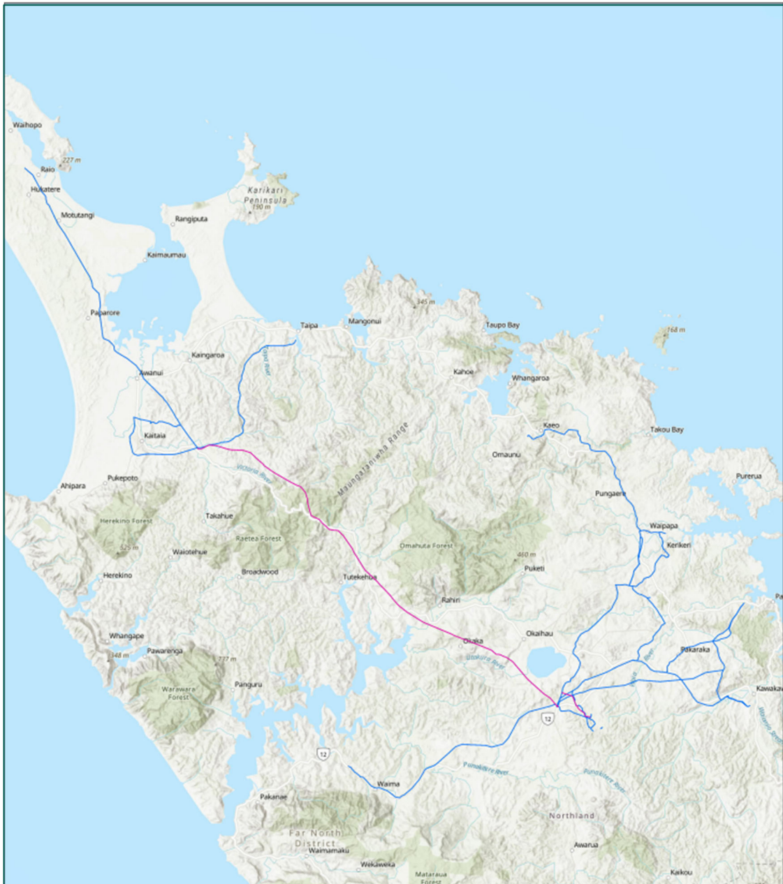
Figure 2 - Top Energy 33kv (blue) and 110kv (pink) network. See full scale version in Attachment 2.
