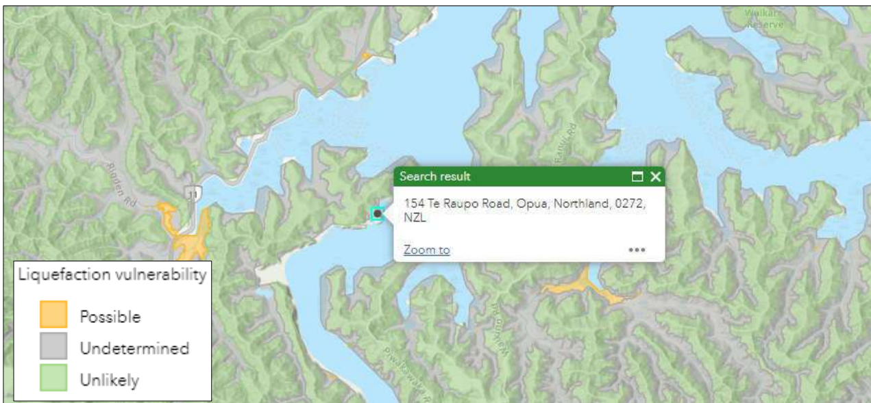
Figure 13: Screenshot aerial view of the subject site from the FNDC on-line GIS Liquefaction Vulnerability Map. Black circle inside cyan square approximately depicts southern end of development location.
