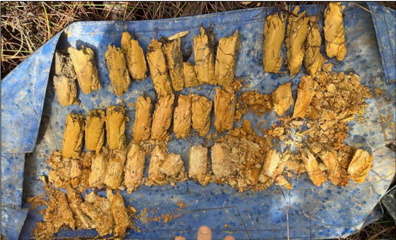
Figure 16: Site photograph of the typical HA soil arisings.
