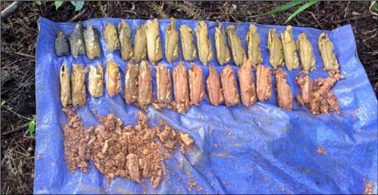
Figure 15: Site photograph of the typical HA soil arisings.
