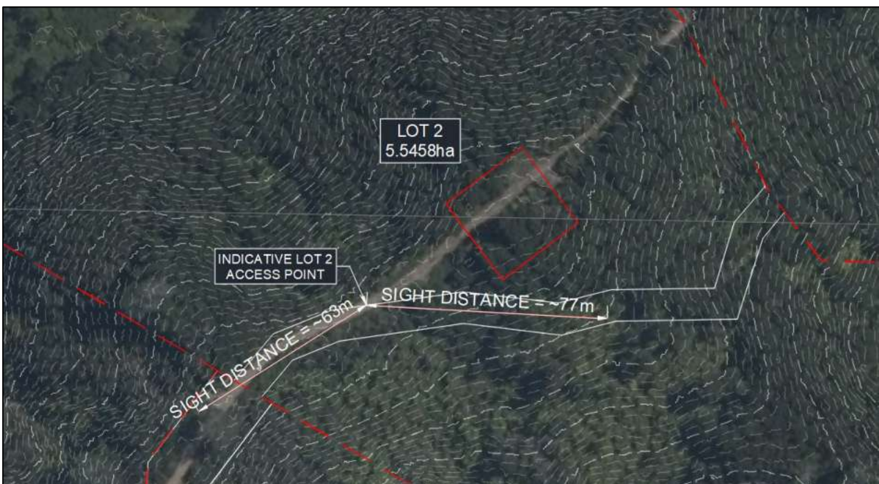
Figure 11: Plan View Indicatively Showing Lot 2's Access Point & Sight Distances.
