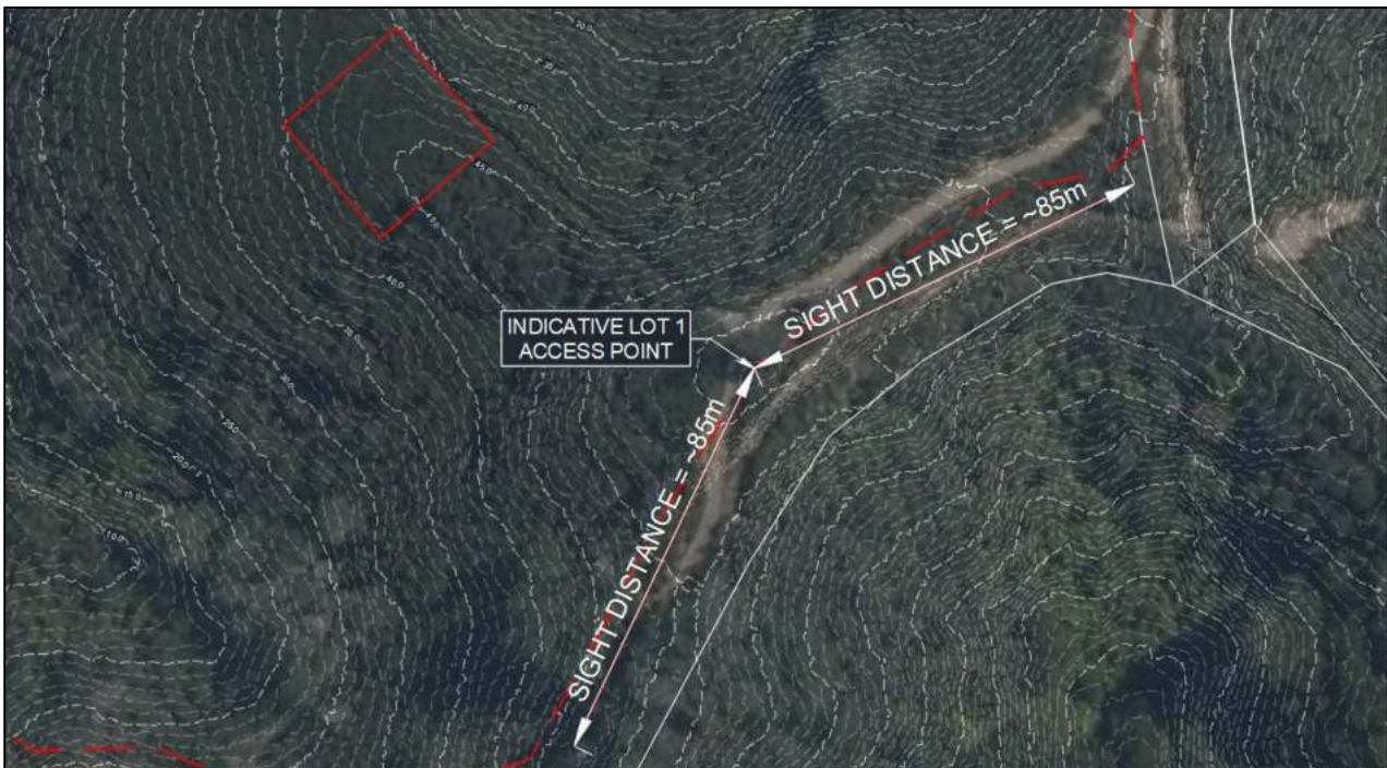
Figure 10: Plan View Indicatively Showing Lot 1's Access Point & Sight Distances.
