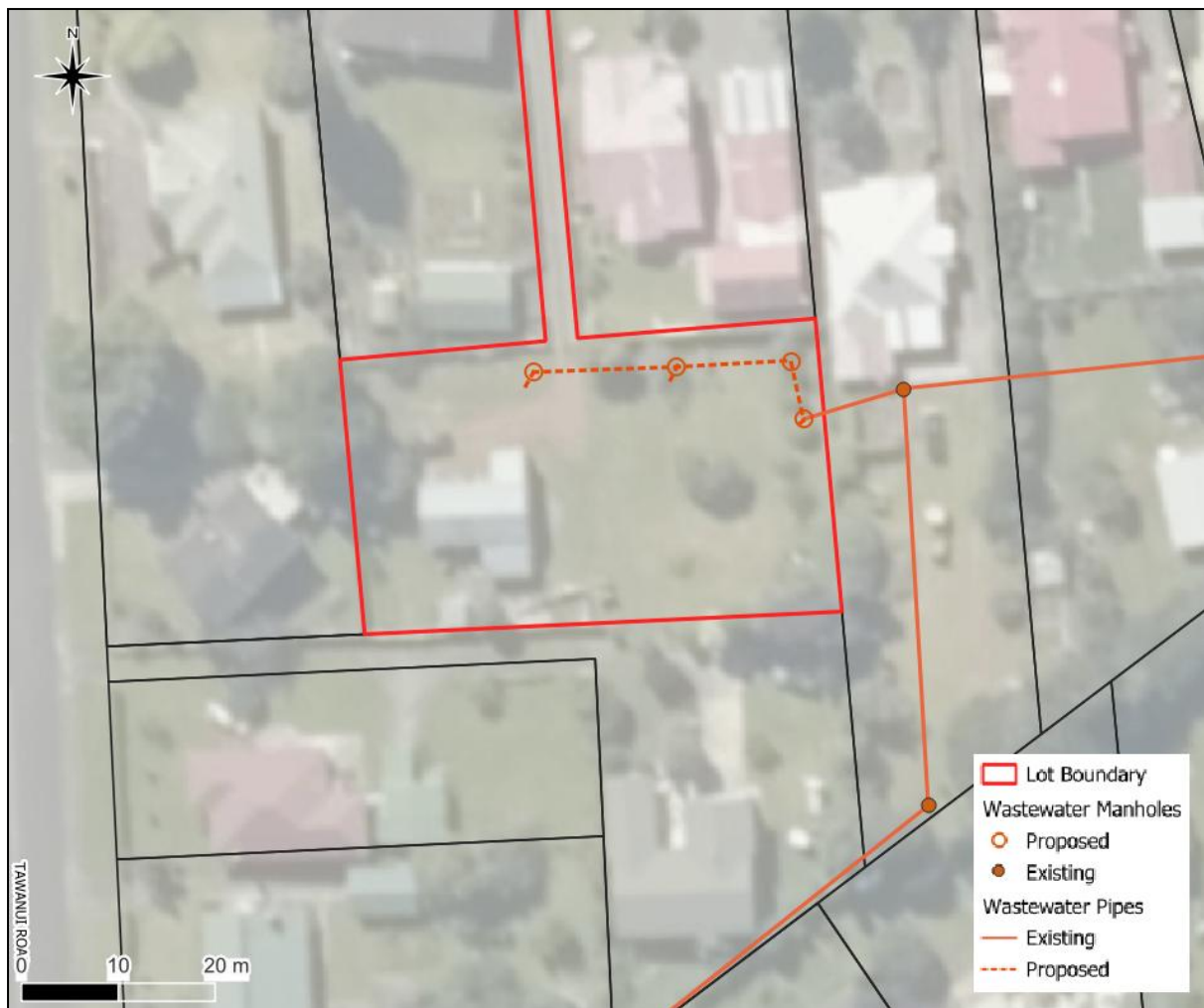
Figure 8: Indicative Wastewater Network Arrangement
