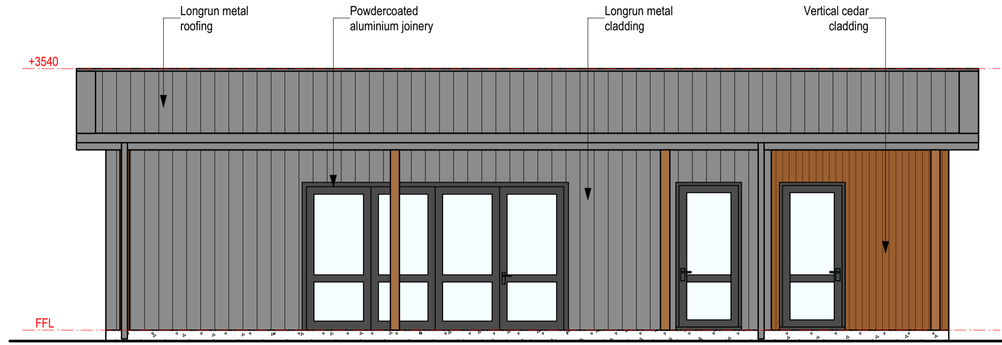
1 Communal laundry - north elevation R-09 Scale: 1:50
