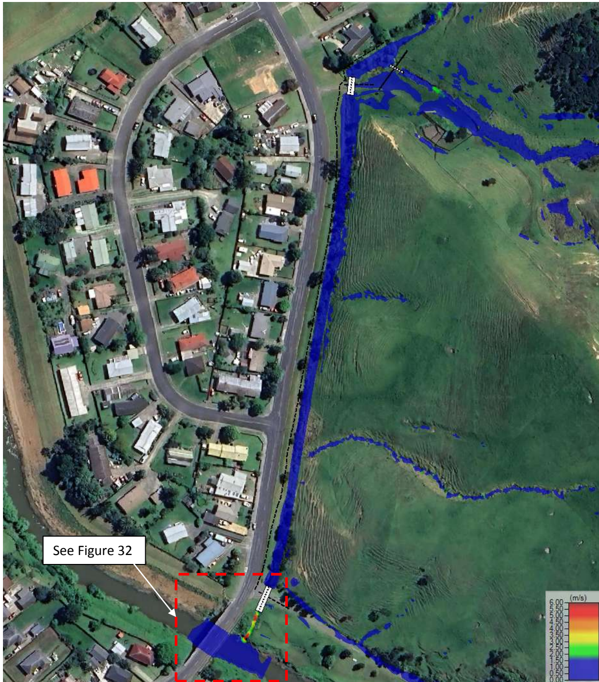
Figure 31. 1% AEP – 1 Hour, Diversion Drain Velocities (no tailwater) Flow velocities shown by banding included in legend, north up the page, not to scale.
