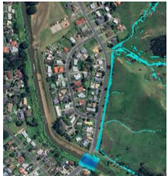
Figure 28. 10% AEP - 12 Hour Flood inundation shown in blue, north up the page, not to scale.
