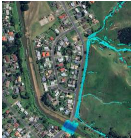
Figure 24. 2% AEP - 12 Hour Flood inundation shown in blue, north up the page, not to scale.
