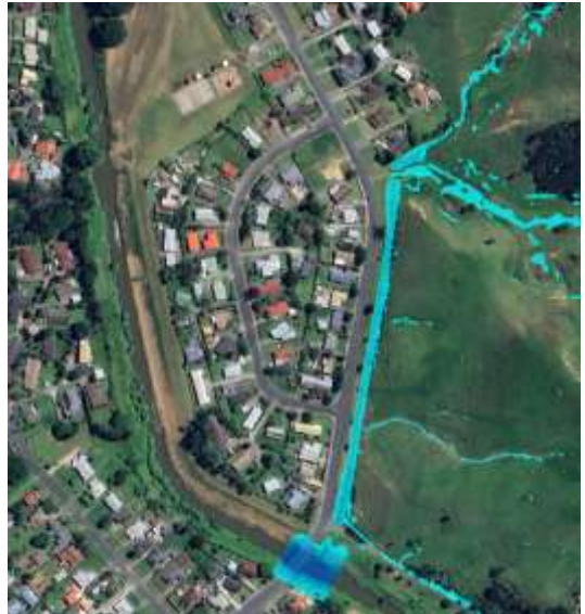
Figure 25. 2% AEP - 24 Hour Flood inundation shown in blue, north up the page, not to scale.
