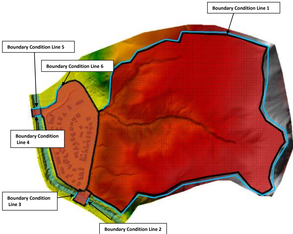
Figure 15. Boundary Conditions Boundary Condition lines shown in blue, north up the page, not to scale.
