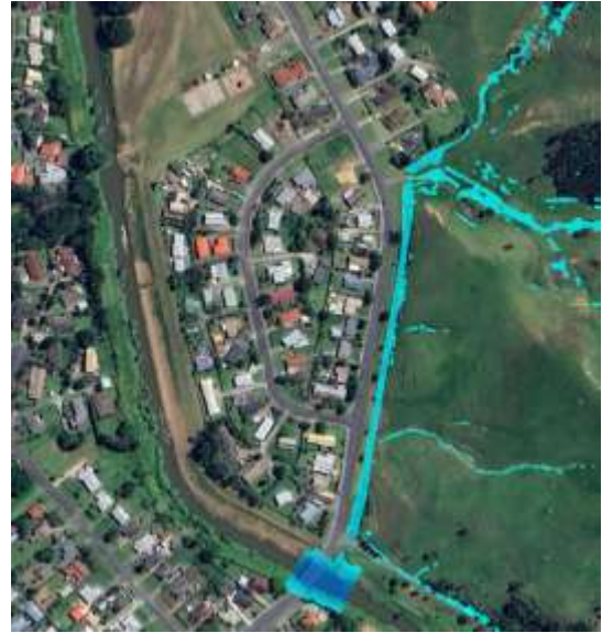
Figure 27. 10% AEP - 6 Hour Flood inundation shown in blue, north up the page, not to scale.
