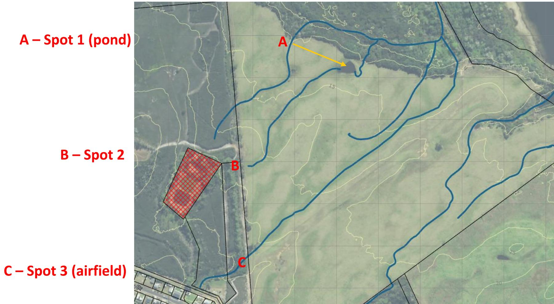
Figure 1: The wastewater treatment plant (red cross hatching), 5m contours (light yellow) and approximate surface (and near surface) water flows in dark blue. The yellow arrow points to the small pond where water quality samples have been taken. Rotokawau Lake (west) is just visible in the top right hand corner.
