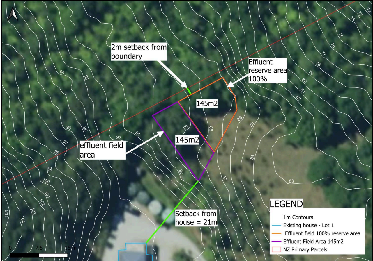
Figure 8 - Effluent Field location plan (Scale 1:400. Map adapted from LINZ Aerial Imagery with NRC 1m contour overlay).
